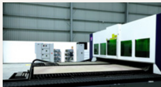
Laser power up to: 20 kW Table size: 16,000 mm x 4,000 mm Cutting up to: 30 mm & beveling up to 45°
