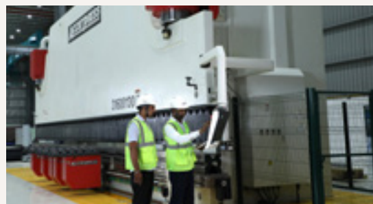
Max press brake: 1,600 tonnes Bending length: 13,000 mm
